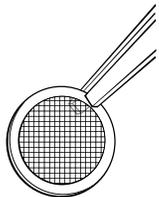
**Electron Microscope (E.M) grid** – These small (less than ¼ inch in diameter) grids are made of copper and nickel and are used to hold specimens that are inserted into a transmission electron microscope (T.E.M). Specimens are placed on top of the grid that has a thin membrane coating on top to keep the specimen from falling through the open areas in the grid.
