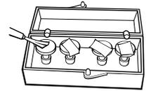
**Sputter Coater** (pronounced – “sputter coat r”) This device is used to prepare specimens that are going to be viewed in a scanning electron microscope (S.E.M.). The thin layer of gold improves the image quality by conducting the extra electrical charge away from the sample. Gold coated images are easier to see because they do not have white streaks and or areas where the specimen cannot be seen.
