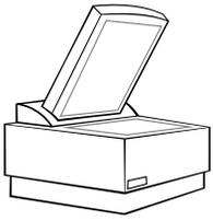
**Phosphor-imaging scanner** (pronounced - “fos for”) – This instrument replaces the need for X-ray film when working with radio active isotopes in molecular biology, genetics, and medical radiography. Instead of using X-ray film developed in chemicals, the exposed imaging plate (phosphor screen) is read using a scanning red-laser system. This instrument looks like a really big flatbed scanner.
