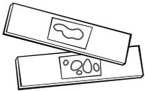
**Microscope** (pronounced – “Mic row scope”) **slide** – Clear glass slides used to view samples under a microscope. Usually microscope slides are used in combination with smaller and thinner glass “cover slips” that protect the sample from damage, or drying out.
