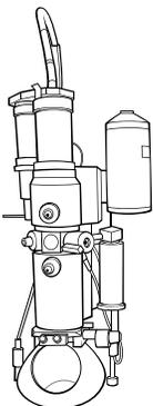
**Electron microscopes** – which use beams of electrons instead of light, are designed for very high magnification usage. Electrons, which have a much smaller wavelength than visible light, allow a much higher resolution. The main limitation of the electron beam is that it must pass through a vacuum as air molecules would otherwise scatter the beam.
