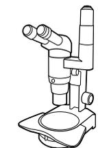
**Dissection** (pronounced – “die section”) **microscope** – Microscopes that are used to look at objects in the range of 1X (twice normal size) to 60X (sixty times normal size). Dissection microscopes have two eye pieces so that the users can judge depth and distance while working with materials and samples.
