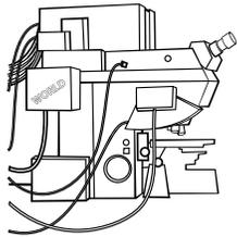
**Scanning-laser confocal microscope** – This light microscope is best used to produce sharp three-dimensional images and allows viewer to see not just surface features, but often all the way through the sample. The microscope scans successively deeper layers of a specimen and then uses a computer to assemble the various images into a single composition. This technique eliminates blurring and scatter common in most light microscopes.
