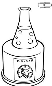
**Magnetic stirrer** (stir plate) – Magnetic stir plates use rotating magnets, or a stationary electromagnet to spin a bar magnet usually coated with a special plastic material that can withstand being submerged in solutions without dissolving or interacting with the solutions. When the bar magnet, also called a flea, is placed in a beaker containing liquid on top of a stir plate the bar will rotate as the magnetic field is increased, or the rotating magnet in the base
