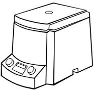
**Microcentrifuge** – Simple centrifuges are used in biology and biochemistry for isolating and separating biomolecules, cell organelles, or whole cells. They vary widely in speed and capacity. Molecular biology laboratories use “microcentrifuges” extensively. These benchtop centrifuges typically accommodate microcentrifuge tubes with capacities from 250  $\mu$ L to 2.0 mL.
