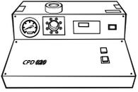
**Critical Point Dryer** – This instrument is used to remove water and fluids from biological samples without damage. Under normal conditions when cells lose large amounts of water the result is cell damage and or drastic change in cell shape, such as when a grape is dried and becomes a raisin. Critical point dryers are able to remove the water from cells, without causing damage or change in cell shape.
